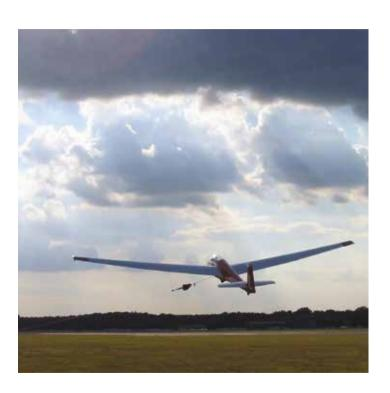
A glider with a 1g stalling speed of 34 knots will stall at about 50 knots during rotation on a winch launch if the rotation rate is 20° per second. The stall speed will be about 45 knots if the rotation rate is 15° per second.
