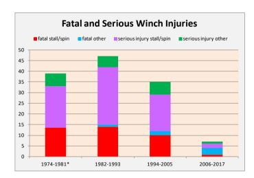
The fatal and serious injury winch accident rate in the last 12 years is a vast improvement on the previous rate but we need to continue to work hard at safe winch launching if the current accident rate is to be maintained and driven even lower.
