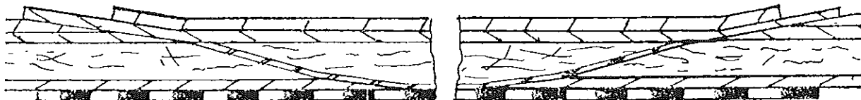
Laminate Outer skin layers Same number of layers as original
