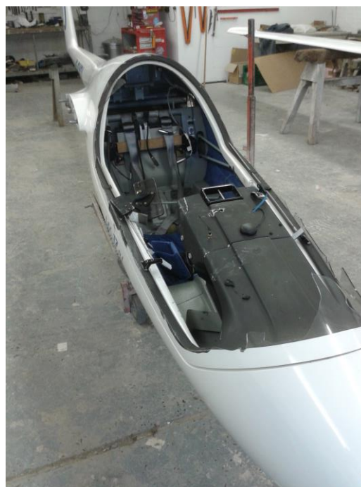
(e) Damage to 170's right cockpit edge and instrument binnacle
