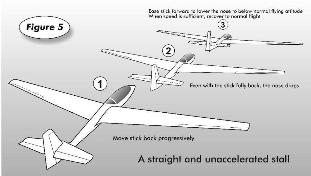
The degree of forward stick movement and the time and height taken to unstall the glider depends on the circumstances of the stall. For example:
