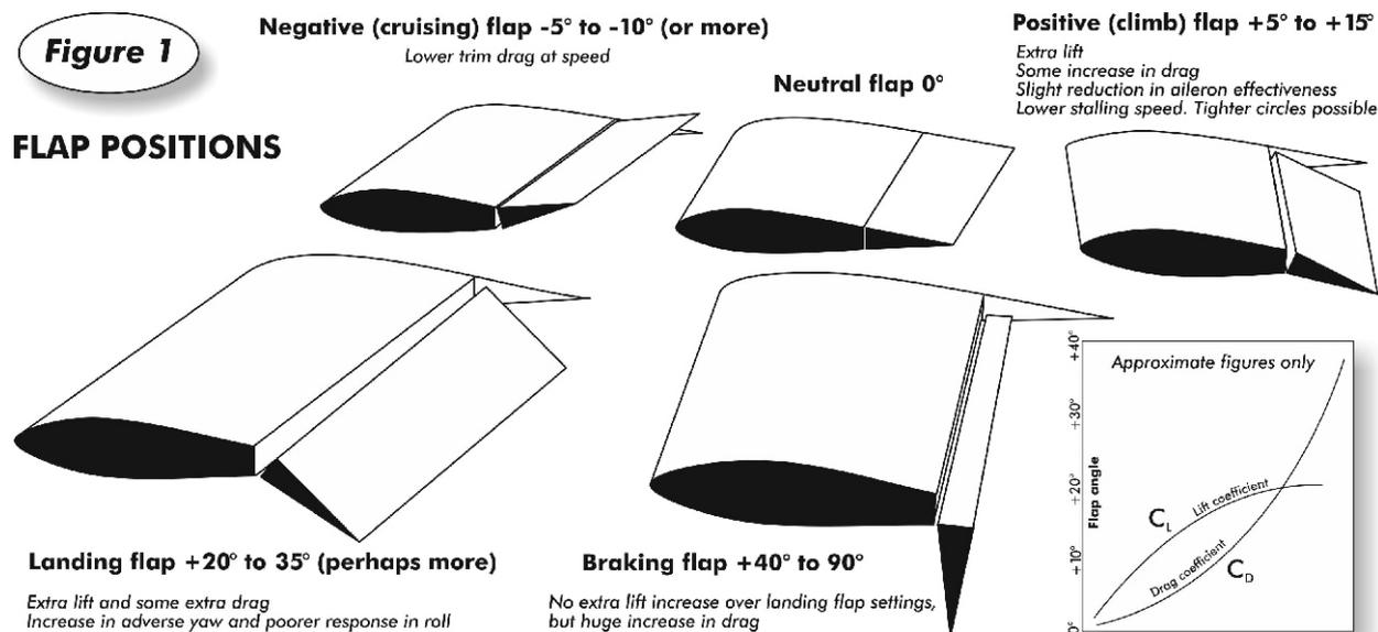
Aerofoil sections optimised for thermalling don't operate efficiently at inter-thermal cruising speeds, and vice versa. Trailing edge flaps address this fundamental problem by giving the pilot the ability to change an aerofoil's camber and characteristics so that it works efficiently over a broader range of speeds than a comparable unflapped section.
