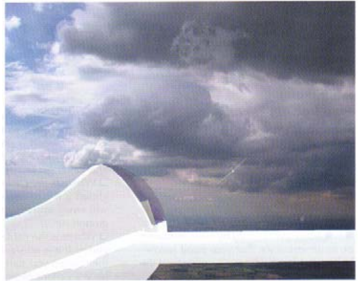
Note the position of the thermalling glider's tail against a point on the horizon; this should be the extent of its turn (all diagrams by Simon Adlard)
