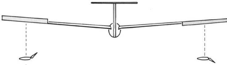
The result is that the aircraft rolls or 'banks' to the left around a line drawn through the fuselage from nose to tail (the longitudinal axis). This is called a movement in the "rolling plane", ie, banking. If you hold the stick to the left you will continue to roll (or bank). If, therefore, you want to alter the angle of the aircraft in the rolling plane, you move the stick to one side, wait until the required attitude is reached, and then centralise the stick to maintain the attitude.
