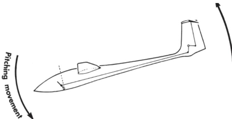
This pitching movement in flight alters the angle of attack of the wings to the airflow and the balance of forces is upset, causing the flight path to change.
