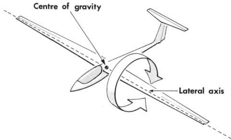
**Remember** - No matter what the attitude of the aircraft is in relation to the ground, the controls always have the same primary effect on the aircraft (unless it is stalled). The ailerons give control in the rolling plane, the elevator in the pitching plane and the rudder in the yawing plane. These planes are referred to the aircraft and not to the earth.
