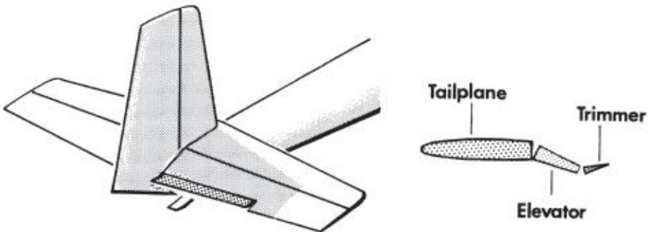
The trimmer is used to relieve the pilot of work in maintaining the required attitude in pitch. If, for instance, the pilot wishes to fly faster, she moves the stick to effect the necessary change of attitude and then, once the speed is steady, adjusts the trim until the aircraft maintains that attitude without any need for pressure on the stick. Remember set the *attitude*, check correct *speed* and then adjust the *trimmer*.
