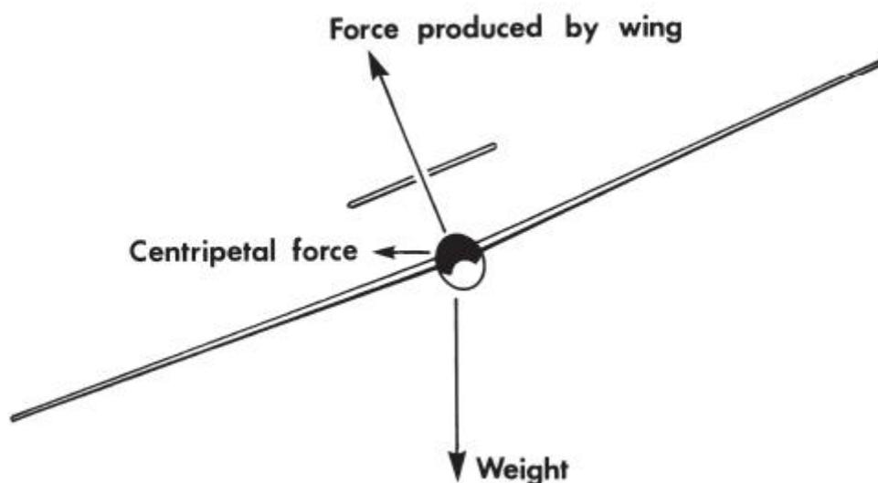
The weight of the aircraft still has to be supported during the turn; in order to do this as well as provide the necessary centripetal force, the total lift must be increased. As explained earlier, the "load factor" is now greater than one.
