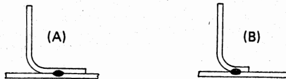
Figure 2 ATTACHMENT OF STRINGERS TO SHEETS
