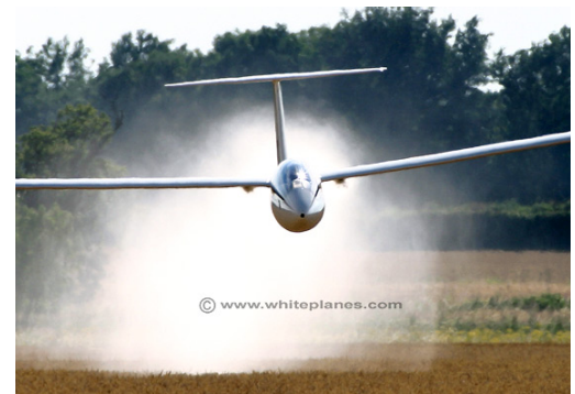
glider dumping water ballast
