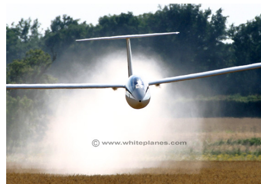
glider dumping water ballast
