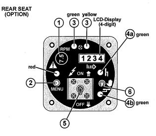
The engine control unit TB 06 is designed for a partially automatic extension and retraction procedure of the power plant for engine operation.
