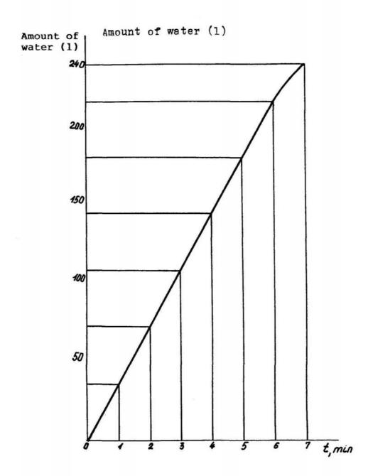
Fig. 5. Dependence of the drained water ballast amount on the drain time.
