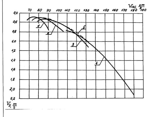
Fig. 2. Drag polar of the sailplane descent rate at the different flap positions (m = 430 kg)
