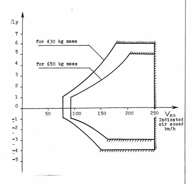
Fig. 7. Dependence of available load factor on the flight speed. Flaps up ( $\sigma_{\rm fl} = 0^0$ ), landing gear and air brakes retracted.
