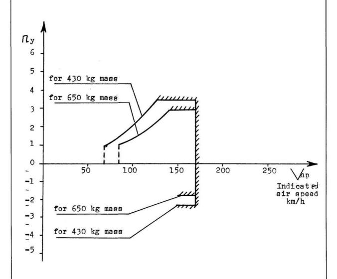
Fig. 9. Dependence of available load factor on the flight speed. Flaps down ( $\sigma_{fl} = 18^{0}$ ), air brakes and landing gear extended
