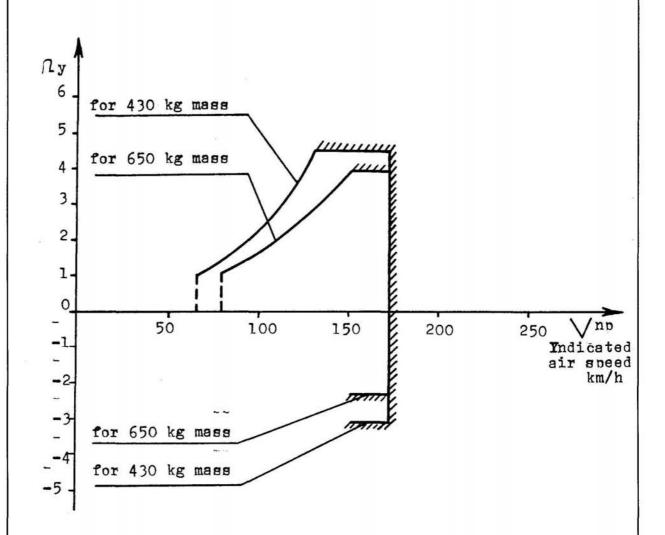
Fig. 8. Dependence of available load factor on the flight speed. Flaps down (  $\sigma_{\rm fl}$  =18 $^{\!0}$  ), air brakes and landing gear retracted.
