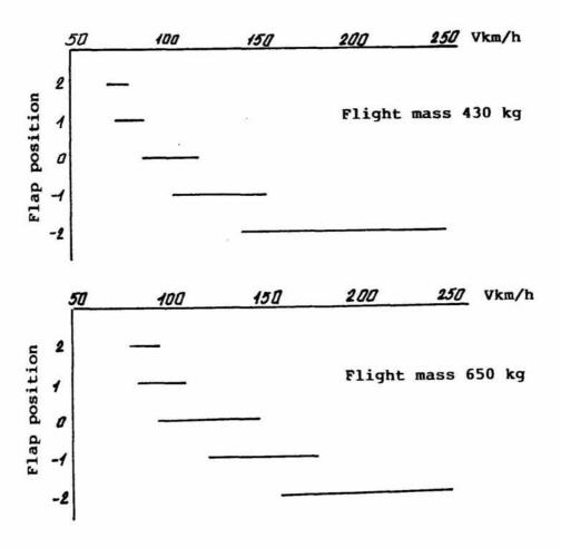
Fig. 4. Dependence of the optimum flap position on the flight speed.
