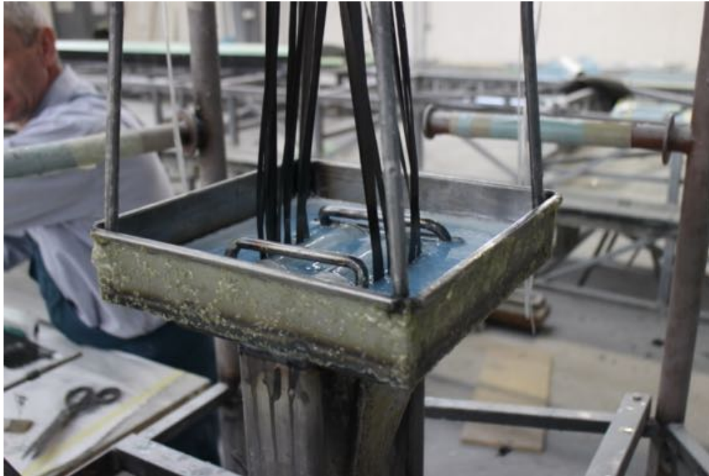
Carbon Rovings being drawn Through a resin bath
