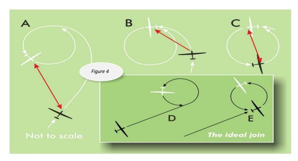
Figure 4 shows how spiralling in ought to work. If you are not in the 'correct' position, you can continue turning outside the other glider's circle until you are. Nevertheless, spiralling in to match circles, speeds, and stay in the correct position, is difficult to do well.
