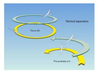
Where relevant, the vertical separation between your glider and the closest should be at least 100'. At that vertical separation, if you are both flying 15m gliders and are steeply banked, one above the other (figure 1), the nominal separation between your nearest wingtips will be just 65 ft, which is close!
