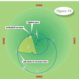
The lift core is at A. Variometer lag means that the strongest lift is not indicated until point B. If the pilot then straightens up C), the glider will be heading almost directly away from the core. The mistake has already been made, so whatever method of counting the pilot uses to decide when to turn again at, say, D, the situation will be worse than it was before.
