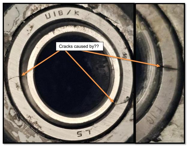
**09 LS3 lower rudder hinge corrosion** (applies to many other LS types) **Advisory** If you see anything like this during an annual/ARC, it's not acceptable to leave it. If treated early the hinge would not have needed changing.
